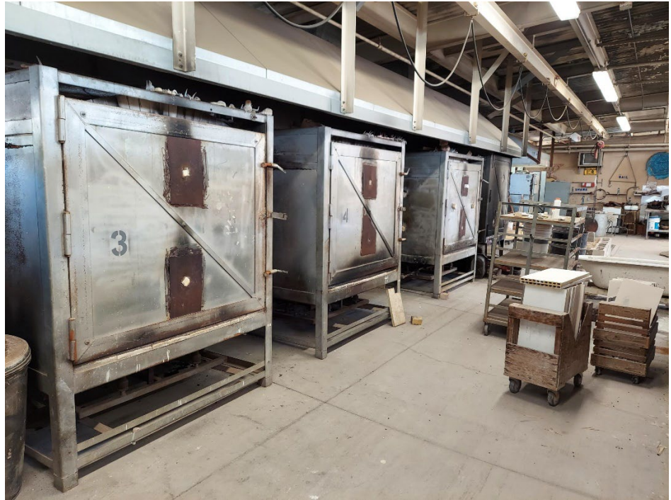
Photograph 1: General view of large kilns needing mechanical advantage to load.
