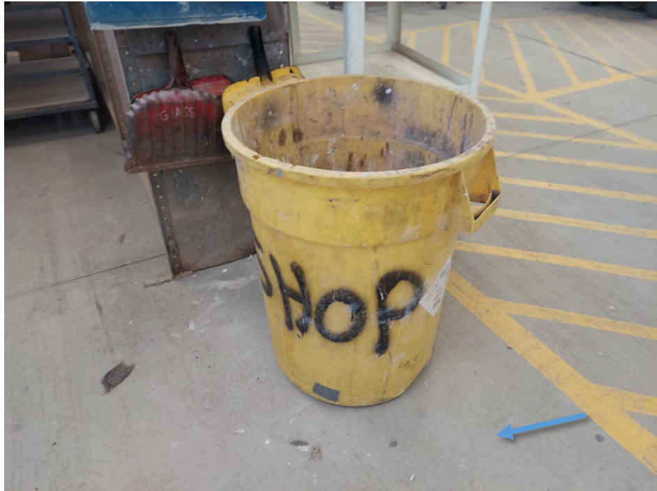
Photograph 11: Large trash can observed in working area, Containers of this size should be replaced with smaller receptacles or handled using mechanical advantage.
