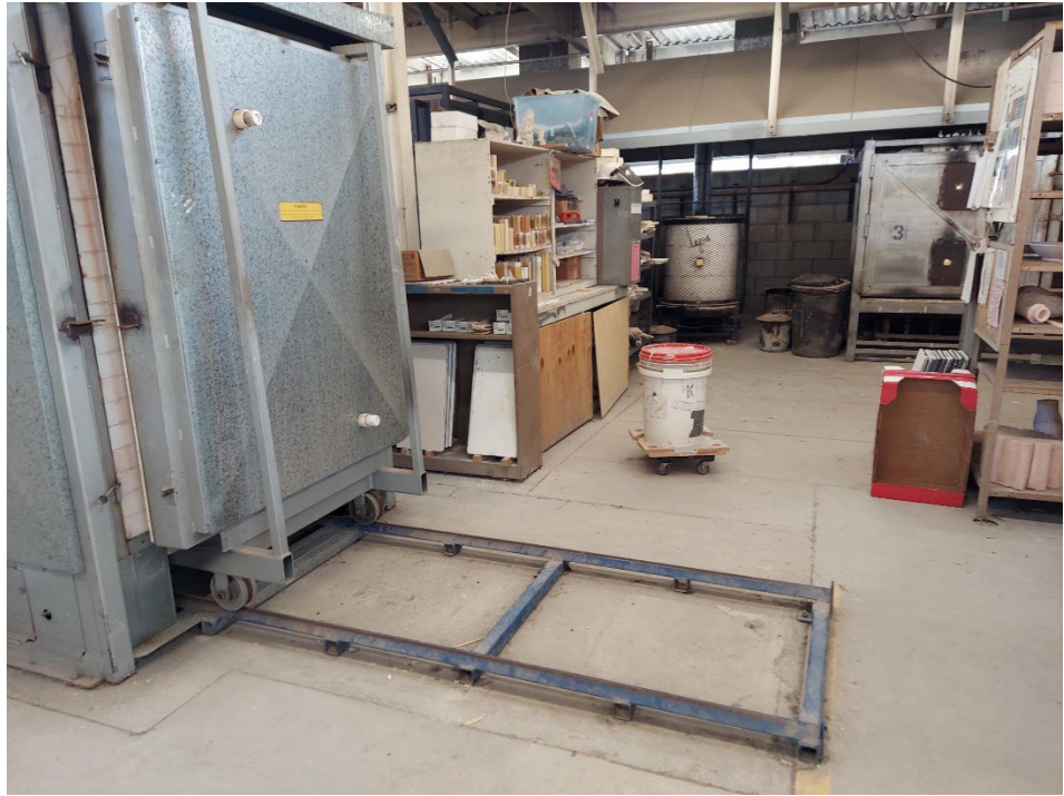
Photograph 7: Tripping hazard requiring high visibility demarcation.
