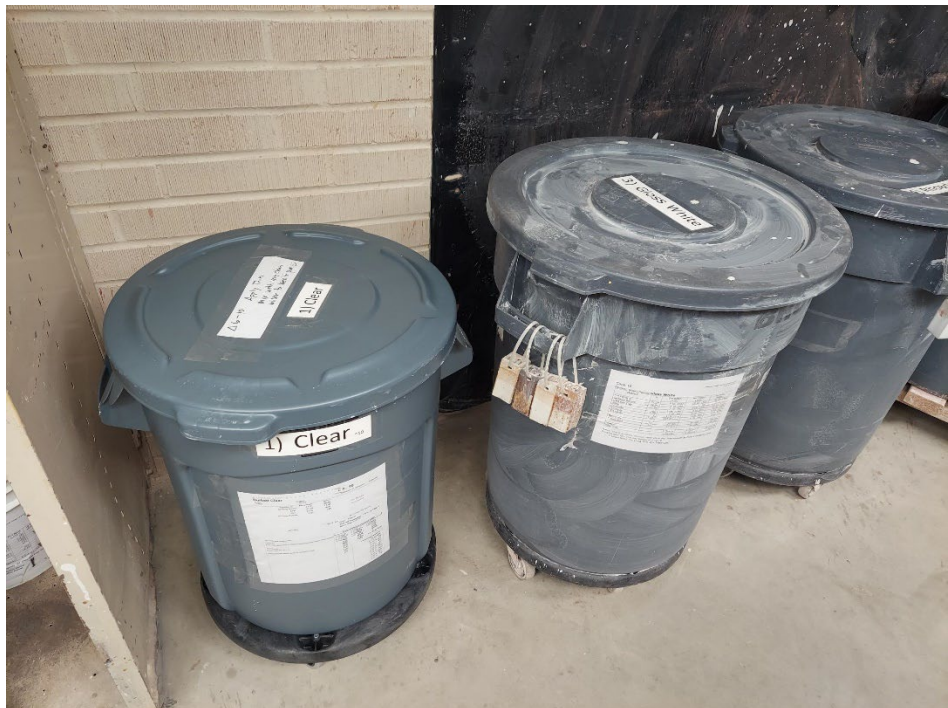
Photograph 12: Two sizes of material containers. Smaller containers are ideal for reducing lifting/handling exposure and are easier to maneuver.
