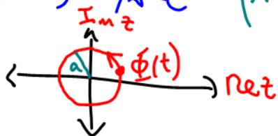
$\underline{\Phi}(t)$  rotates ccw around circle of radius  $a$  in complex plane.
