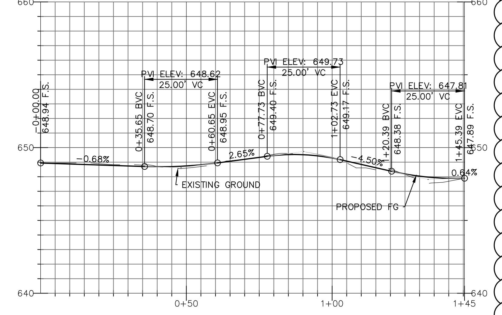
PROFILE VIEW: ALIGNMENT - F HORZ. SCALE: 1"=20' VERT. SCALE: 1"=4'
